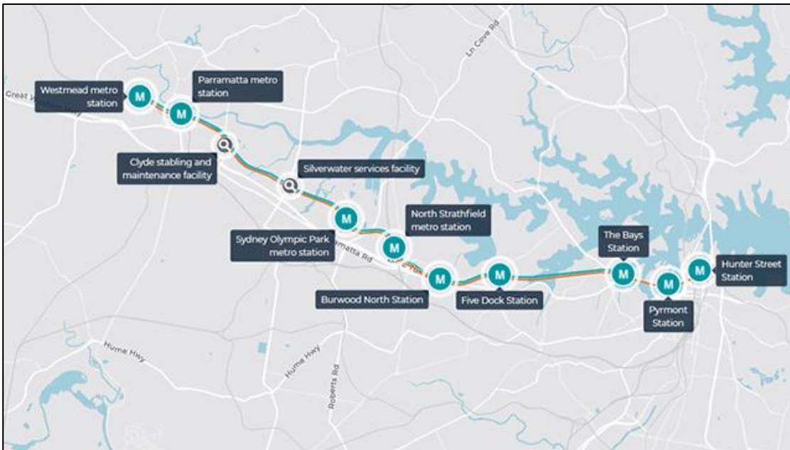
Figure 6 Sydney Metro West alignment (Source: Sydney Metro, 2022)
